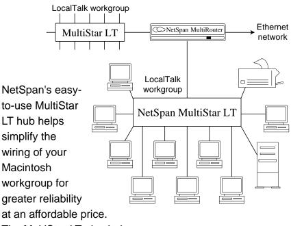
The MultiStar LT also helps you easily connect your LocalTalk workgroup to an Ethernet network through NetSpan's MultiRouter EN/LT.
